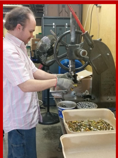
Matthew Spurbeck crimping valves for MTE Hydraulics
