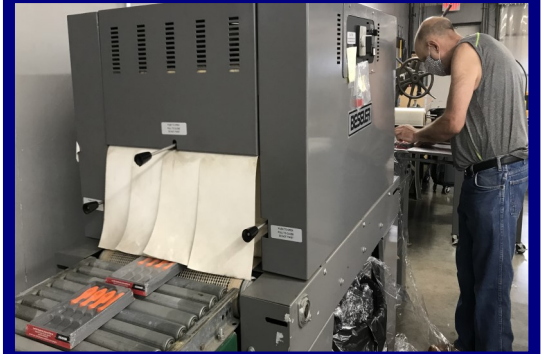
John is putting Snap-on Tool kits into the shrink wrap machine. These sets are ready for shipping.
